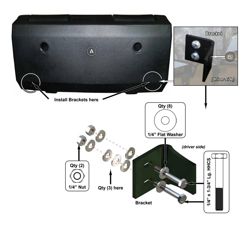
Disassemble Latch and Go's and install to Cargo Box. **DO NOT TIGHTEN NUTS COMPLETELY**.
